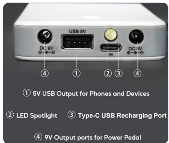
Figure 10 A pedal-style power bank can supply both 5 V (USB hub) and 9 V (merge unit) from one battery.
