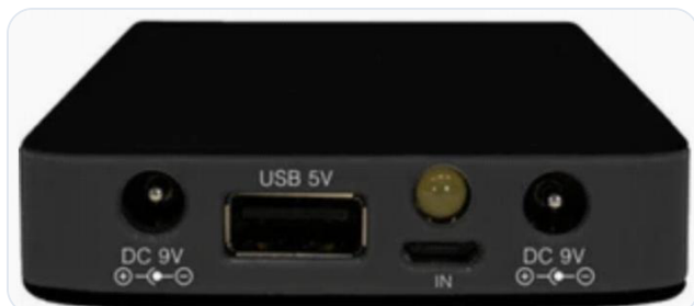
Figure 11 A pedal power bank can power the CME MIDI merge (DC 9 V) and the powered USB hub (USB 5 V) at once — leaving the USB-C or 5-pin MIDI port free to feed your DAW or sound module.
